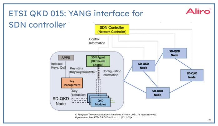
In the diagram above, the yellow box represents the quantum network controller, and the blue boxes below represent the quantum network nodes. One of the blue boxes on the left has been magnified to show its internal structure.
