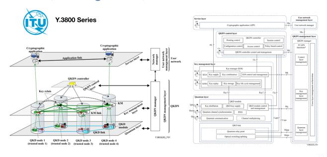
The figure on the left in the graphic above is taken from ITU-T Y.3803. It shows the layers of a secure communications network.
