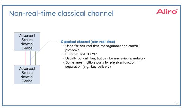
The control protocols are used to control various aspects of the entanglement-based network. A small subset of these control protocols are extremely hard real-time, in the sense that they must be synchronized down to the nanosecond level. However, most of the control protocols are not hard
