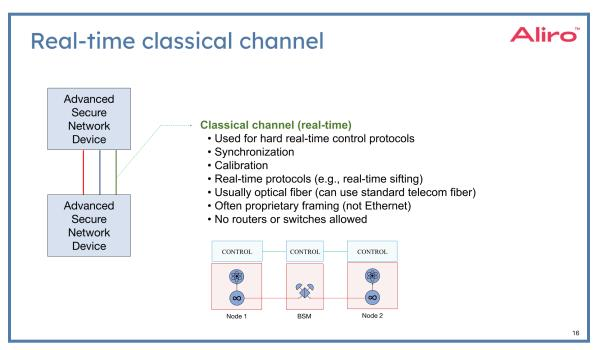
Above is one possible mechanism for implementing elementary entanglement generation. In this example, the source on the left (Node 1) and the source on the right (Node 2) generate photons that need to arrive at the bell state analyzer in the middle (BSM) at exactly the same time, down to the nanosecond level. This requires extremely precise clock synchronization protocols. The entanglement generation protocol is non-deterministic in the sense that multiple attempts are needed to get a
