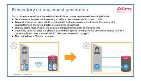
The first step of this meet-in-the-middle technique is to generate an entangled pair consisting of at least one photonic qubit at each of the two neighboring nodes. This is achieved with an entanglement source. Then a photonic qubit from each of the two entangled pairs is transmitted via optical fiber to a probabilistic Bell state measurement station, consisting of a beam splitter and two single photon detectors.
