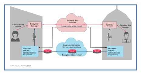
Entanglement-based key generation utilizes distributed entanglement to generate a shared secret key between end users. This method has information-theoretic security, which means regardless of how strong an adversary's computational resources, whether classical or quantum, the key cannot be broken. This is especially important considering the impending nature of Q-Day. Learn more about Q-Day and how organizations can prepare for it in this on-demand webinar "What is Q-Day?"
