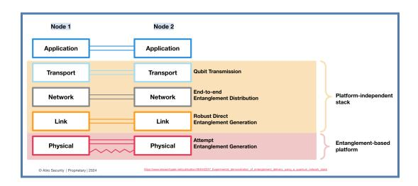
Each layer of the stack will be examined through the example of using an entanglement-based advanced secure network and the BBM92 protocol for entanglement-based key generation. While specifics of all the protocols used in the stack could differ, this example will still give a good overview of how an entanglement-based secure network operates.
