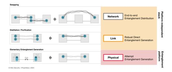
These processes, or protocols, align with the bottom three layers of the entanglement-based network stack. EEG is a physical layer protocol, where entanglement is distributed between neighboring nodes. Entanglement purification is a link layer protocol, creating robust entanglement generation. Entanglement swapping is a network layer protocol, crucial to creating end-to-end entanglement across distance.
