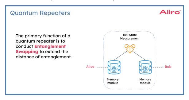
Once those entanglements are established, the entangled photons can be emitted to a Bell state measurement station to perform the entanglement swapping operation. The entanglement swapping operation essentially creates a direct entanglement between Alice and Bob in this example.
