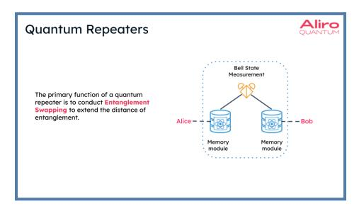
Once those entanglements are established, the entangled photons can be emitted to a Bell state measurement station to perform the entanglement swapping operation. The entanglement swapping operation essentially creates a direct entanglement between Alice and Bob in this example.
