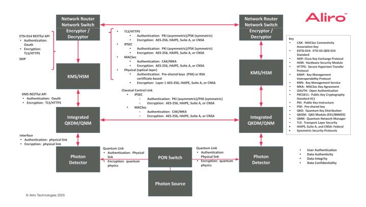
In the protocols mapped \ above, at the very top are the network routers and network switches. The encryptors / decryptors are there also. Most often in today's modern networking technology, those services are all integrated into a single device.
